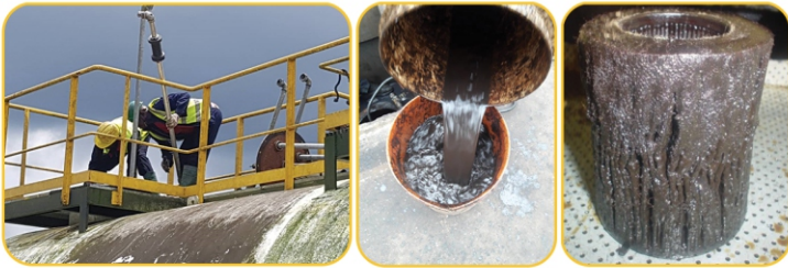
dirty fuel causes equipment breakdown
